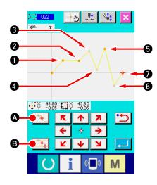
Input the breakpoint in the ordinary sewing. For the ordinary sewing, the point to be inputted is determined according to the kind of element immediately before the point where DECIDING POINT button Select ORDINARY SEWING (function 022) or 022, and input points (), (2), (5) and (7) with DECIDING POINT button (3) and points (3), (4) and (5) with PASSING POINT button
