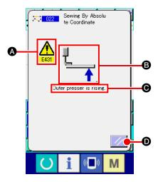
When an error occurs during motion of the body input mode, the error screen is displayed.
