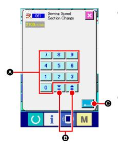
① Display the sewing speed section change setting screen. Press SEWING SPEED SECTION CHANGE button in the standard screen or select and execute SEWING SPEED SECTION CHANGE (function code 061) . in the code list screen, the sewing speed section change setting screen is displayed.
