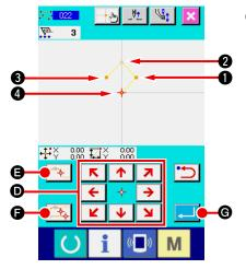
Press MOVE key  $\leftarrow \rightarrow \bigcirc$  in the coordinate input screen, and the needle position moves in the specified direction. When DECIDING POINT button  $\frown$  is pressed, the shape point of
