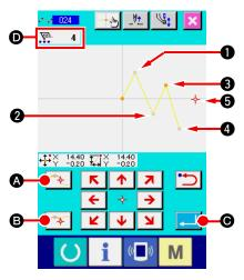
The breakpoint is the point where two points of the shape point of spline sewing are overlapped, and shows the termination of one spline curve. The point where ENTER button \_\_\_\_\_ () and DECIDING POINT button \_\_\_\_\_ () are pressed with the input of spline sewing becomes the breakpoint.
