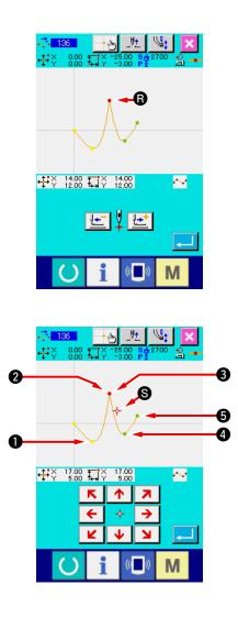
When you desire to move point (B) to point (S), the result will be changed by selecting either shape point of rear (2) or front (3).
